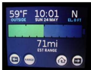
Sample of battery ½ depleted.
