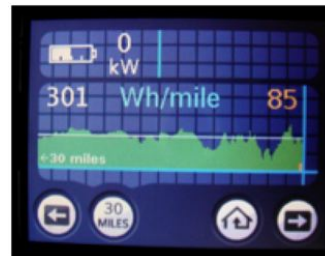
But add some highway miles and we can spend 0.301 kWh/mile or more.
